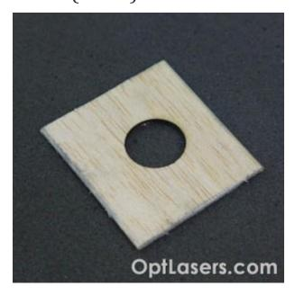
Material: Balsa Thickness: 2mm Speed: 25mm/s
