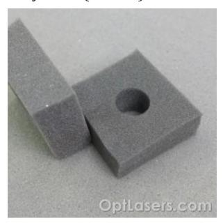
Material: Polyfoam Thickness: 24 mm Speed: 5mm/s
