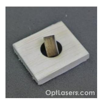
Material: Balsa Thickness: 10mm Speed: 22,5mm/s
