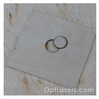
Material: Plywood Thickness: 1,08mm
