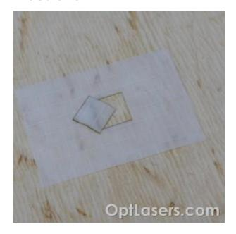
Material: Plastic foil Thickness: 0,2mm Speed: 8mm/s
