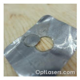
Material: Lead foil Thickness: 0,05mm
