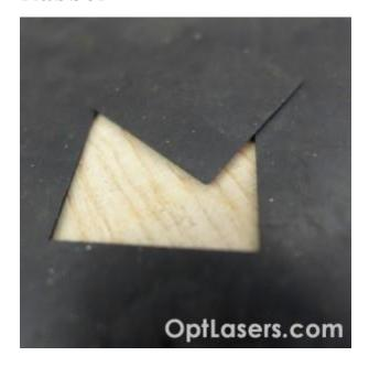
Material: Rubber Thickness: 0,5mm Speed: 15mm/s
