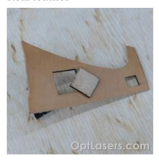
Material: Real leather Thickness: 1,7mm Speed: 5mm/s
